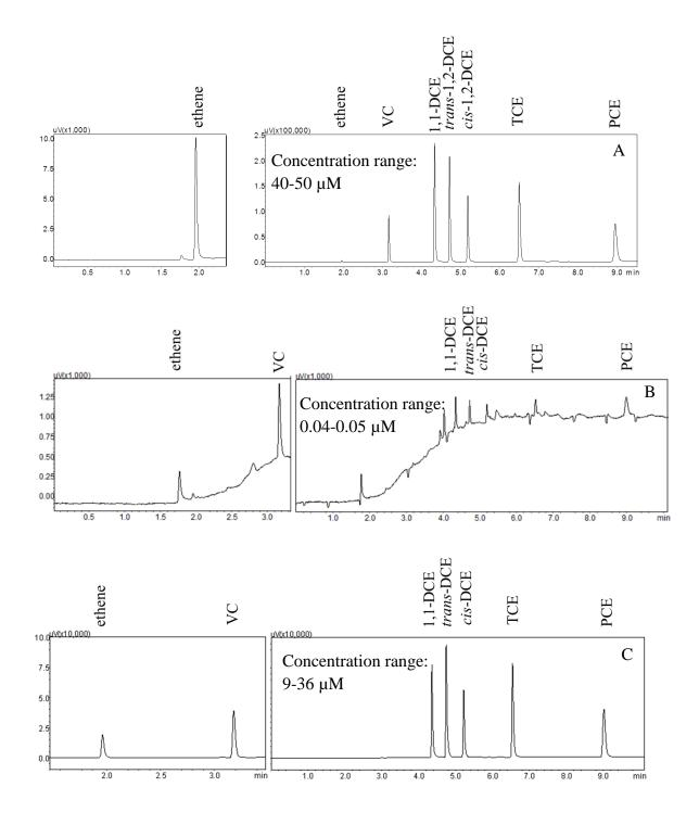
Figure 1. Example chromatogram in DI water for (A) upper linearity values (Table 1) and (B) near the MDLs (Table 1), and in (C) spiked groundwater at the recovery concentrations listed in Table 2.
