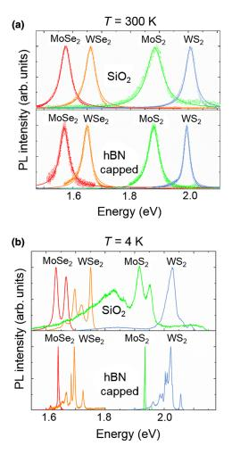
FIG. 2. (a) Typical PL spectra for different TMDC MLs at T = 300 K when deposited directly onto SiO<sub>2</sub> (top) and when capped with hBN (bottom). The excitation density is  $1 \ \mu W/\mu m^2$ . (b) Same as (a) at T = 4 K.
