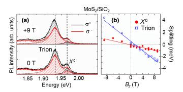
FIG. 5. T = 4 K. ML MoS<sub>2</sub>/SiO<sub>2</sub>/Si. (a) Typical PL spectra for an acid-treated, uncapped MoS<sub>2</sub> ML at selected values of the applied magnetic field. A multiple-Lorentzian fit is employed in order to extract the Zeeman splitting of both neutral and charged exciton (trion) lines, shown in (b). Valley Zeeman splitting as a function of the applied field  $B_z$ . Landé g factors of  $g_X = -1.9 \pm 0.2$  and  $g_T = -6.6 \pm 0.2$  are found.
