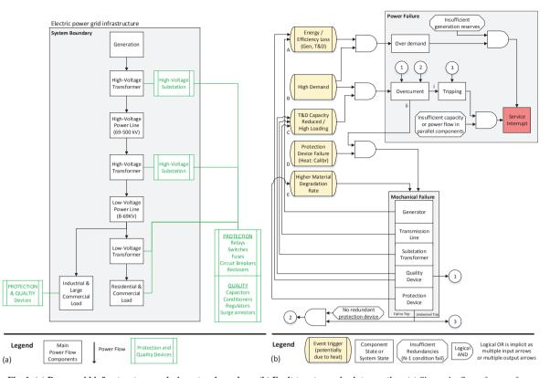
Fig. 1. (a) Power grid infrastructure analysis system boundary; (b) Fault tree to service interruption. (a) Shows the flow of power from generation to load through system components and identifies the analysis system boundary inclusive of major power-flow components including: generation, transmission, substation transformers, and load. Changes in performance of protection and power quality devices are not analysed.
