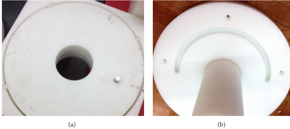
FIGURE 4: (a) Stationary donut-shaped component that rests on the shipping drum; (b) bottom of the RIC that rests and slides on the component shown left.
