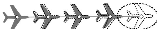
Figure 4. Illustration of prediction compared to measurement with a low entropy and ultimately low information target. Predictions at each track point are represented by the dashed outlines. Actual measurements are shown in the filled-gray planes. The last track point shows the prediction and model mismatch covariance or uncertainty contour. In this illustration, our constant velocity model is well matched to the benign target. As a result, the deviation from prediction at each measurement is small, and for a fixed revisit period as illustrated here, little information is learned through spectral use.
