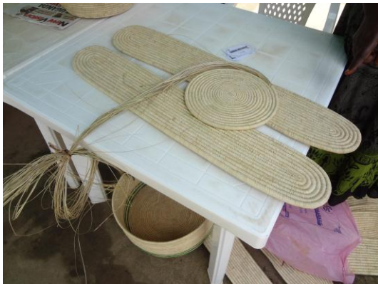
Figure 5. (Left) Woven turbine blades are being completed by a women's group in Uganda using locally dried plants. (Right) A technical student at St. Joseph's Technical Institute in Fort Poratal, Uganda makes a hand cranked electricity generating device out of Legos in class.
