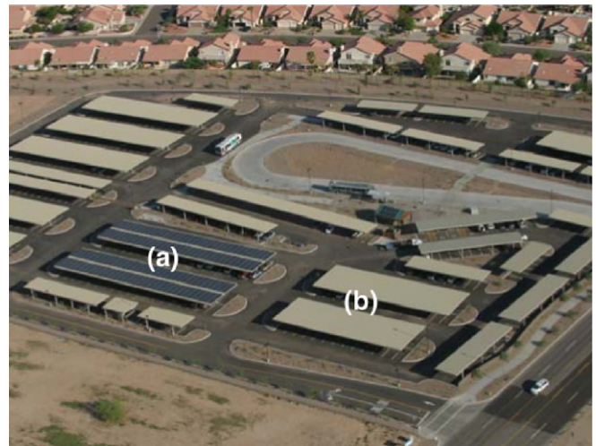
Fig. 6. Aerial view of the subject research site for PV canopy coverage shows (a) PV modified parking canopies and (b) conventional parking canopies, Phoenix, Arizona.
