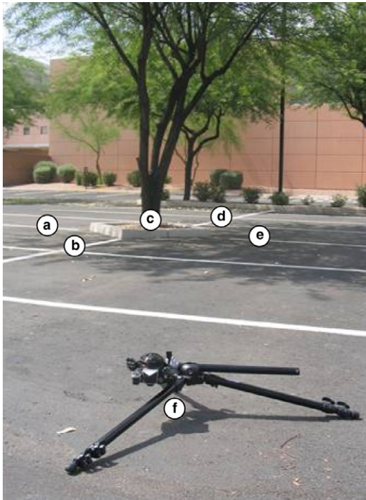
Fig. 1. Image shows the controlled parking utilized for the urban forestry research including camera equipment setup (foreground) and approximate thermocouple locations (background): (a) west edge of canopy cover, (b) south edge, (c) base of tree, (d) north edge, (e) east edge and (f) fully exposed pavement surface.
