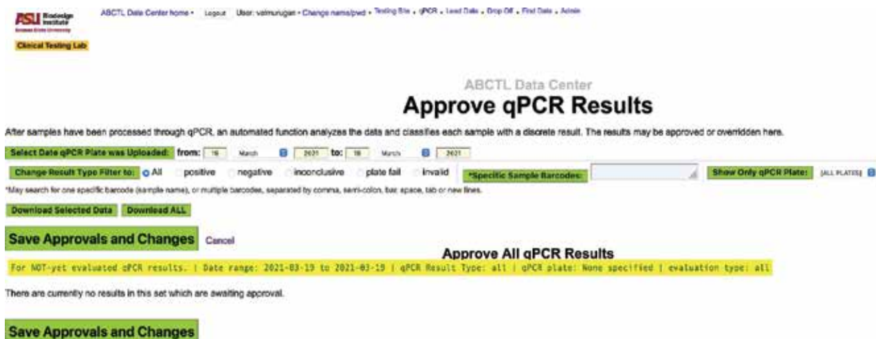
Figure 4. Murugan, V. (2021). The interface of COVID DB. COVID-19 test results can be filtered and accessed by selecting the radio button of the desired test result category. The user (lab director) can also view COVID-19 test results within specific time frames by modifying the "Select Date qPCR Plate was Uploaded" parameters. From ABCTL information technology.
