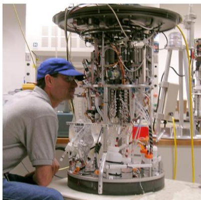
Figure 1. Environmental sampler processor (ESP) developed at MBARI(Courtesy of MBARI http://www.mbari.org/ESP/esp_2G.htm )
