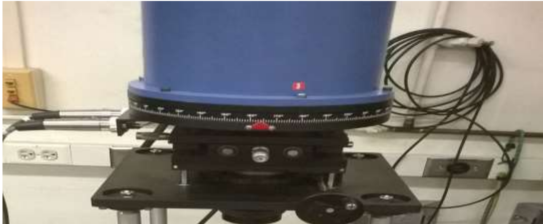
Figure 3. Rotatable head drive of VSM
