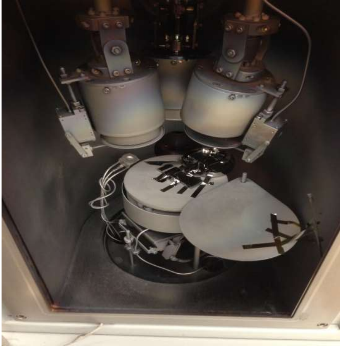
Figure 11 Sputtering with field in easy axis direction angles of 30-60 degrees The magnetic direction is parallel to the near to far direction. One is at the center of the stage (~25 degree). The other is put at the far edge of the stage (~60 degree).
