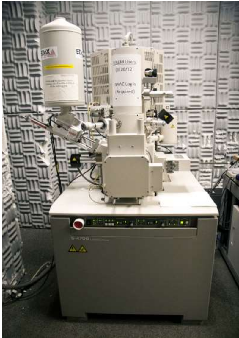
Figure 6. Hitachi S-4700-II FESEM measurement system. Courtesy: asu.edu
