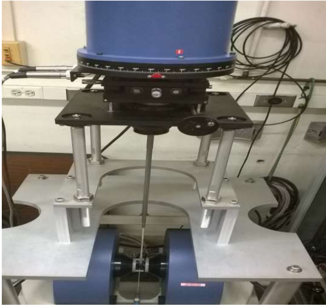
Figure 4 VSM set up with sample inserted and gauss meter enabled
