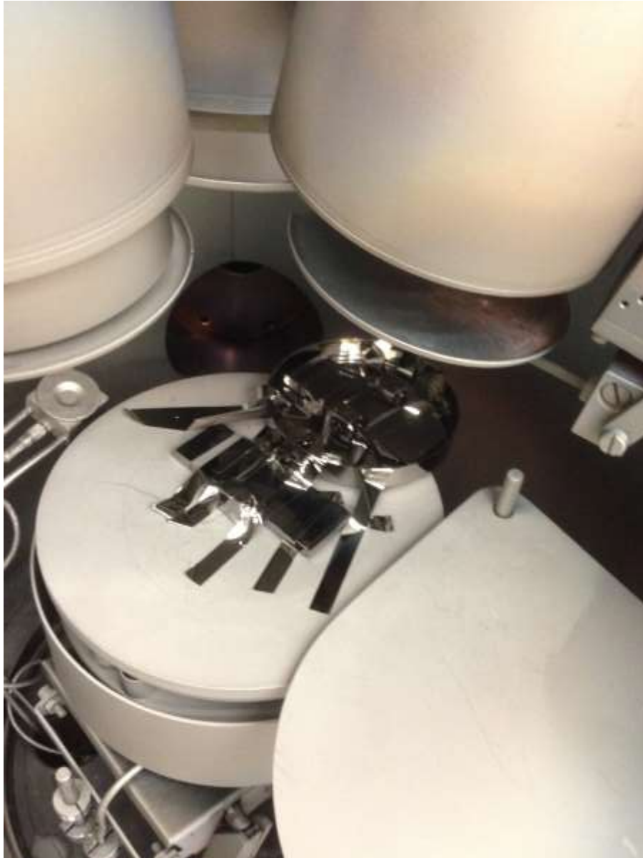
Figure 8. Sputtering with presence of magnetic field during sputtering
