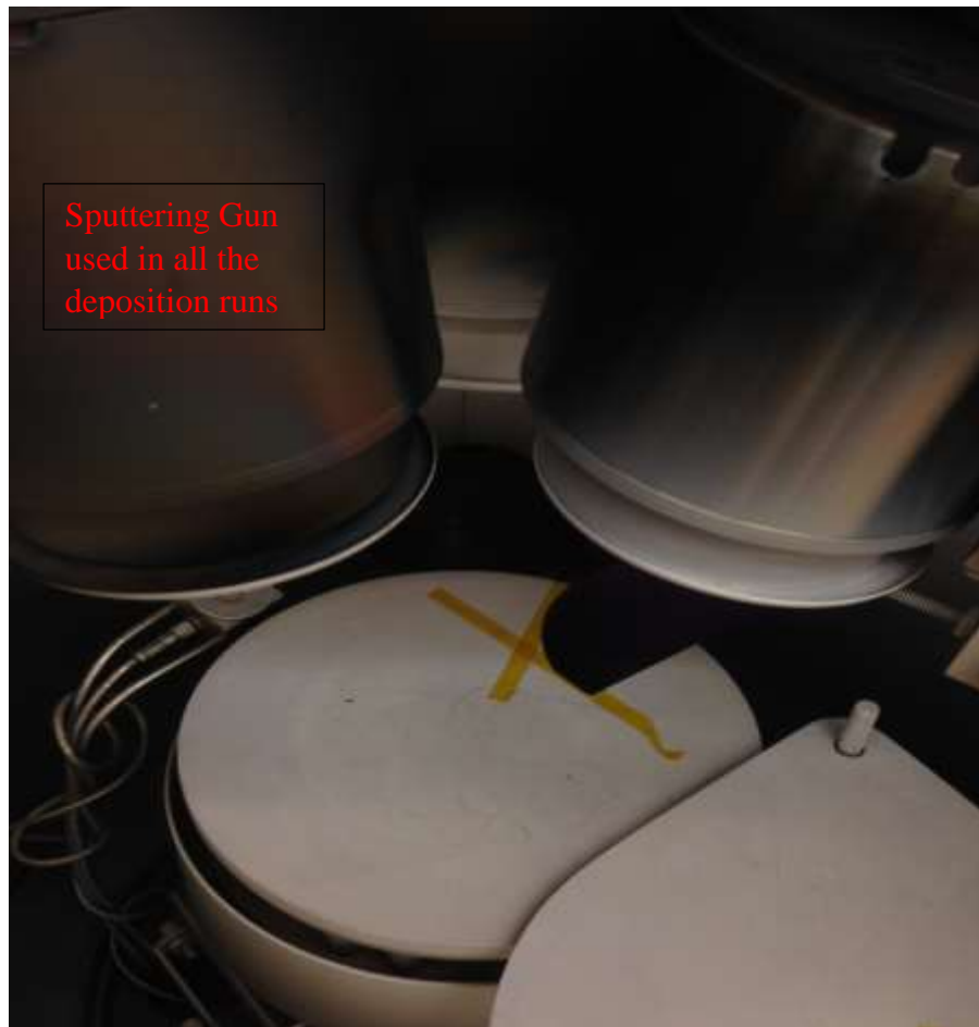
Figure 2 Images of sputtering system set up for oblique sputtering method
