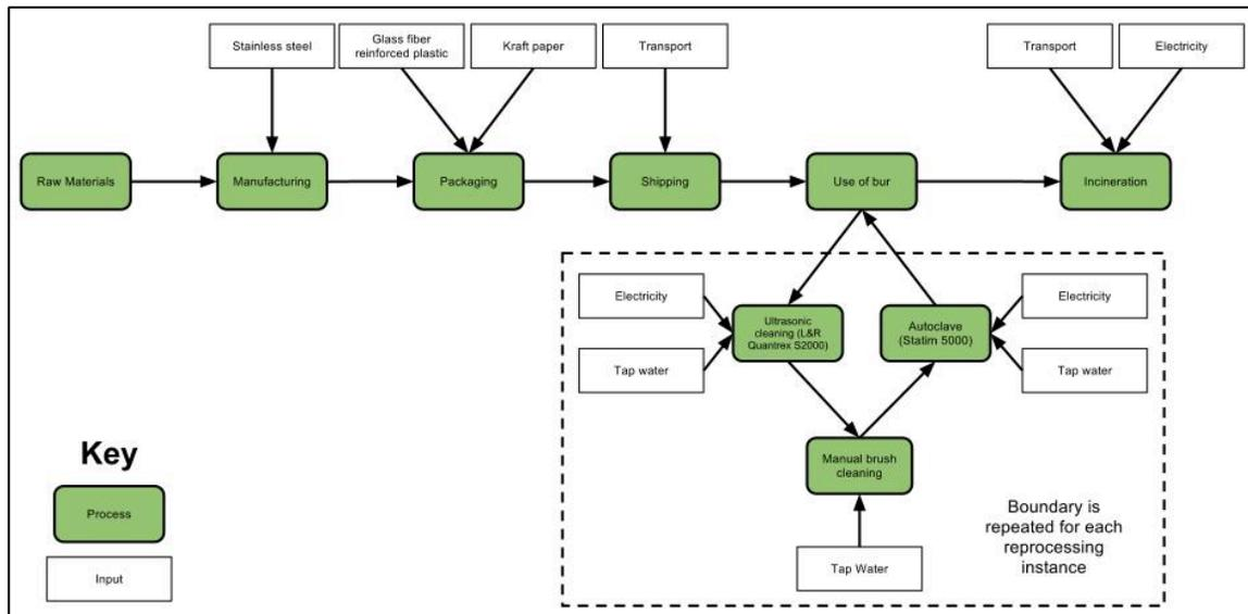
**Figure 2: System boundary showing processes included in the LCA.**
