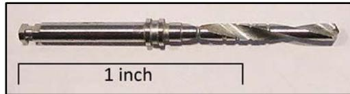
Figure 1: **Diagram of 2.00mm Internal Irrigation Pilot Drill**
