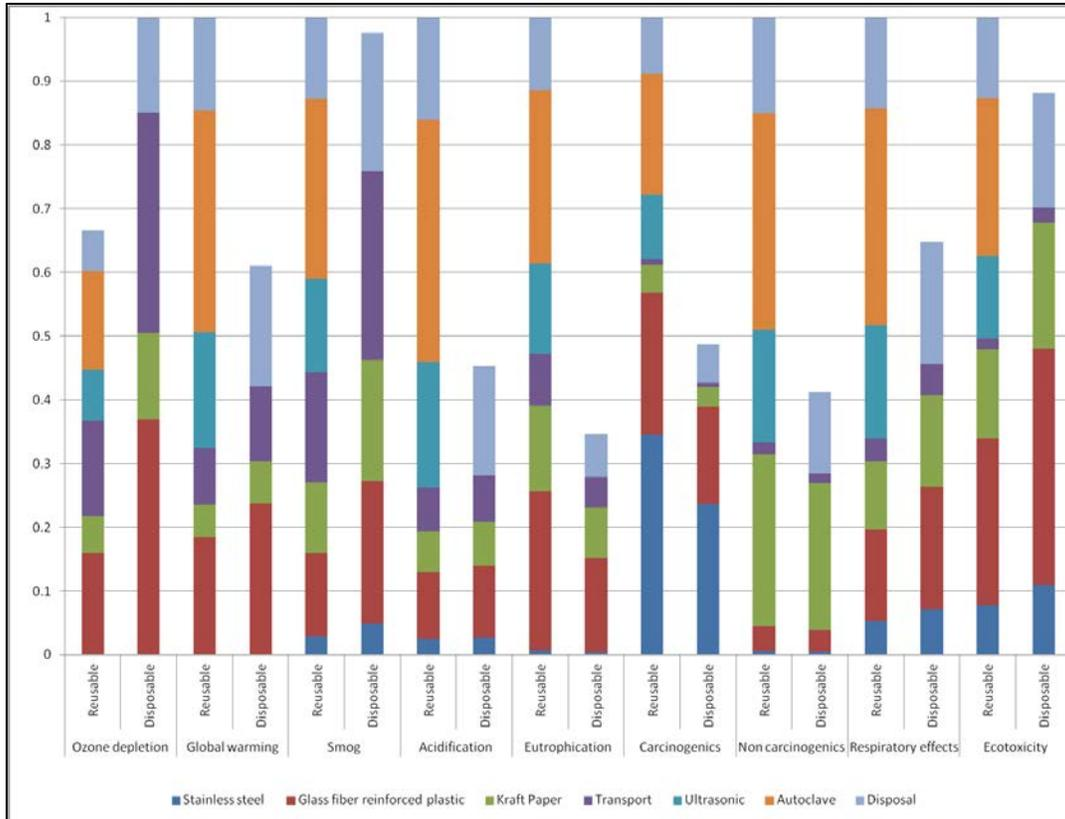
**Figure 6: Worst-case scenario for 30 disposable burs versus 1 bur reused 30 instances**
