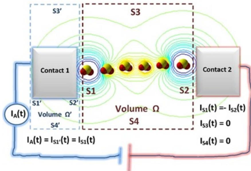
**Figure 1:** A two terminal device with a correct selection of the simulation box  $\Omega$  that allows a correct computation of the flux of particles and the electric flux on  $S_1$ ,  $I_{S_1}(t)$ , so that it coincides with the measured current in the ammeter, i.e.  $I_{S_1}(t) = I_A(t)$ .
