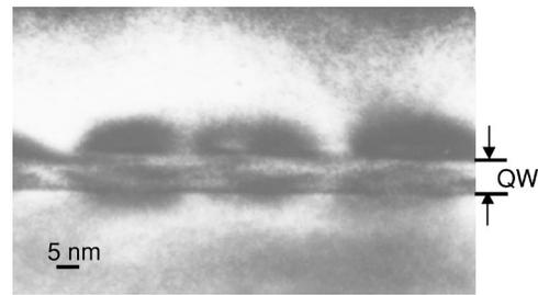
FIG. 2. Dark field electron micrograph showing cross section of an InGaAs/GaPAsSb/InGaAs QW structure. The total well region layer thickness is 9.0 nm.
