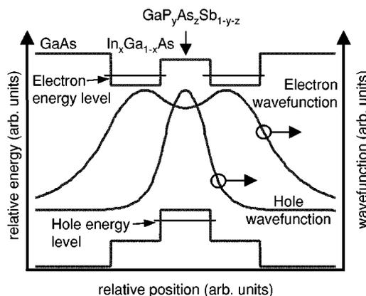
FIG. 1. Schematic band-edge diagram of InGaAs/GaPAsSb/InGaAs type-II QW embedded in GaAs. Schematic electron and hole wave functions are also shown.
