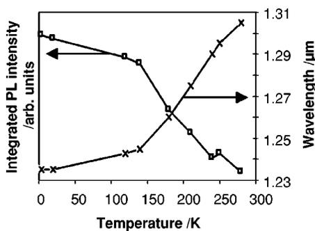
FIG. 4. Temperature dependency of the integrated PL intensity and the peak PL wavelength of sample A at an excitation density of 50 W/cm<sup>2</sup>.
