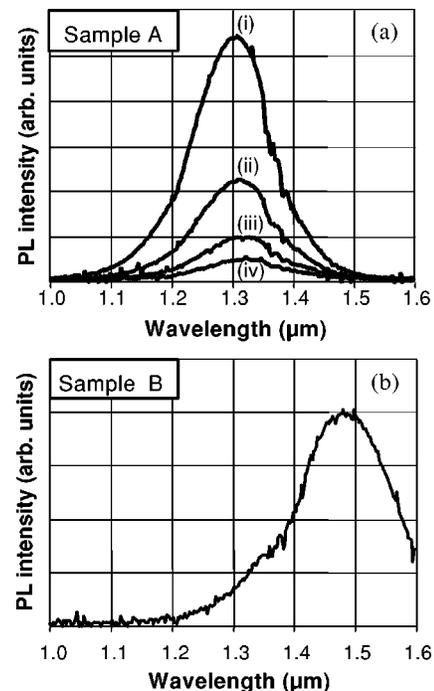
FIG. 3. Room temperature PL spectra of two different InGaAs/GaPAsSb/InGaAs QW structures embedded in GaAs. (a) Sample A at excitation densities of (i)  $1000 \text{ W/cm}^2$ , (ii)  $250 \text{ W/cm}^2$ , (iii)  $100 \text{ W/cm}^2$ , and (iv)  $50 \text{ W/cm}^2$ . (b) Sample B at an excitation density of  $1000 \text{ W/cm}^2$ .
