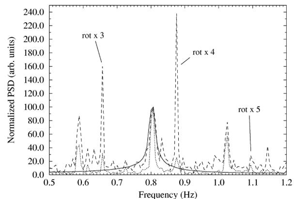
FIG. 4. Comparison of the growth frequency peaks (normalized) for three different measurement methods: (solid line) specular spot intensity, no rotation, (dashed line) integrated intensity along the line perpendicular to the substrate through the specular spot during rotation, (dotted line) FWHM along the line perpendicular to the substrate through the specular spot during rotation.
