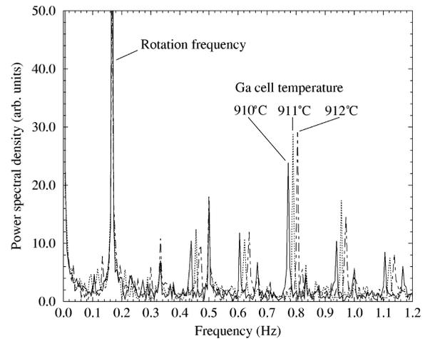
FIG. 3. Frequency spectra of FWHM measurements at three different growth rates, but identical rotation frequency. The measurement time was 180 s.
