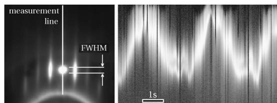
FIG. 1. Measurement geometry and raw signal measured from a rotating substrate. Growth oscillations are measured by determining the FWHM of the specular spot perpendicular to the substrate surface.
