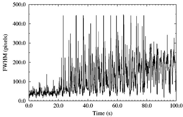
FIG. 2. FWHM of the specular spot perpendicular to the substrate as a function of time in units of CCD pixels. Growth starts at 20 s and terminates at 80 s.
