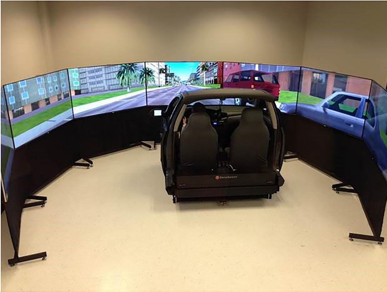
**Fig 1. The driving simulator.**
